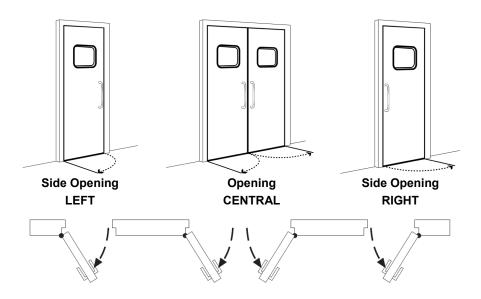
Side opening swing door (one leaf) or middle (two leaves). These can be manual or automatic with the incorporation of a surface motor group. If they are manual, each leaf can make sweep of up to 180°.
