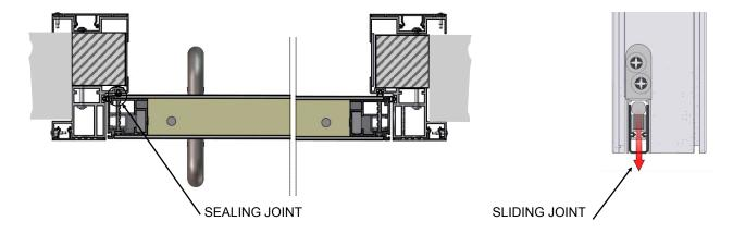
In facilities where the swing door is installed between two rooms where there is difference in pressure, we recommend the door be planned and installed so that the positive pressure always acts in the direction of the door's closing, which helps to keep it in the closed position.
